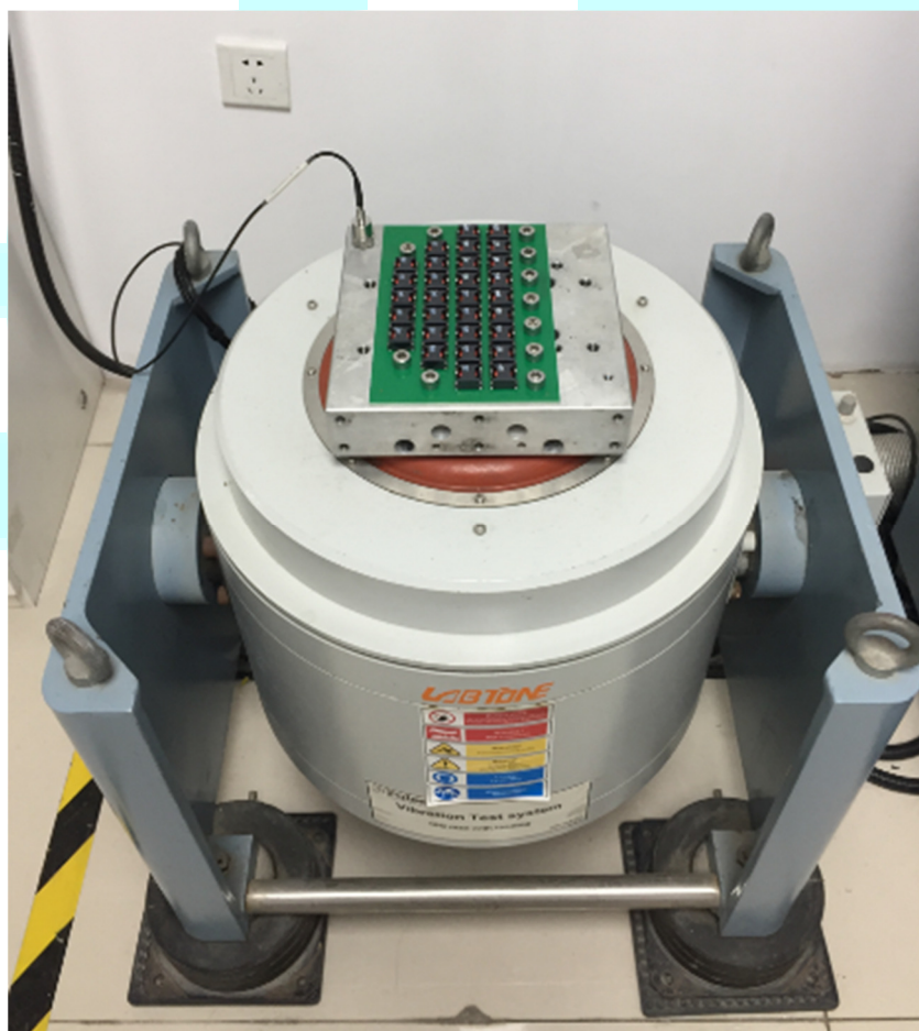
Fig. 2 Vibration Test (X axis)
