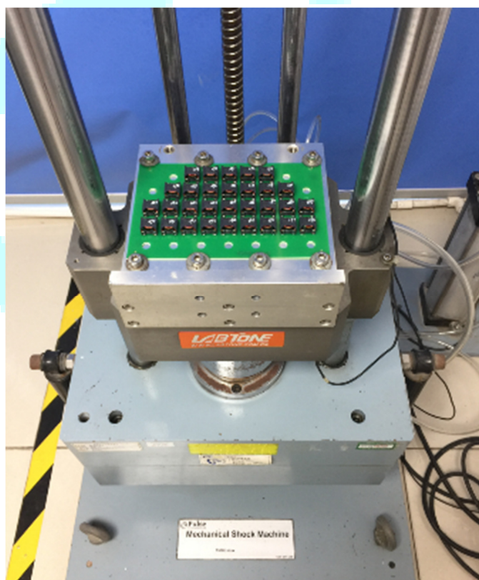
Fig. 2 Mechanical Shock Test (X axis)
