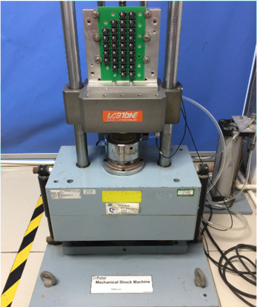
Fig. 4 Mechanical Shock Test (Y axis)
