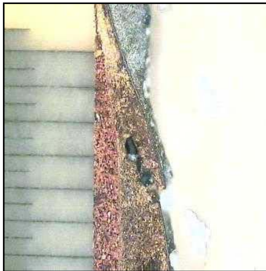
FlexiSafe capacitor post flexure Conductive epoxy stress relief
